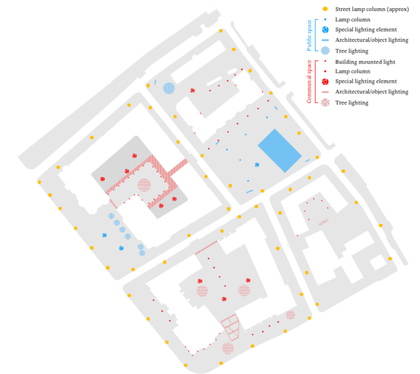
Figure 7 Indicative Street Light Layout (Landscape Design and Access Statement, EAST Architects)
